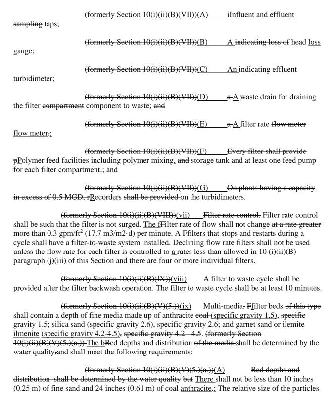
shall be such that hydraulic grading of the material during backwash will result in a filter bed with pore space graded progressively from coarse to fine in the direction of filtration (down).
