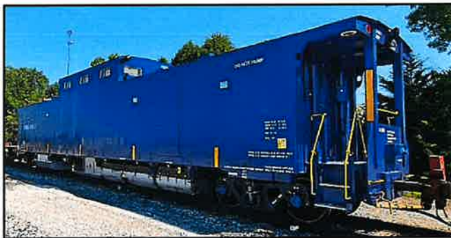
NNPP Rail Escort Vehicle (Identified by "DODX" reporting mark)
