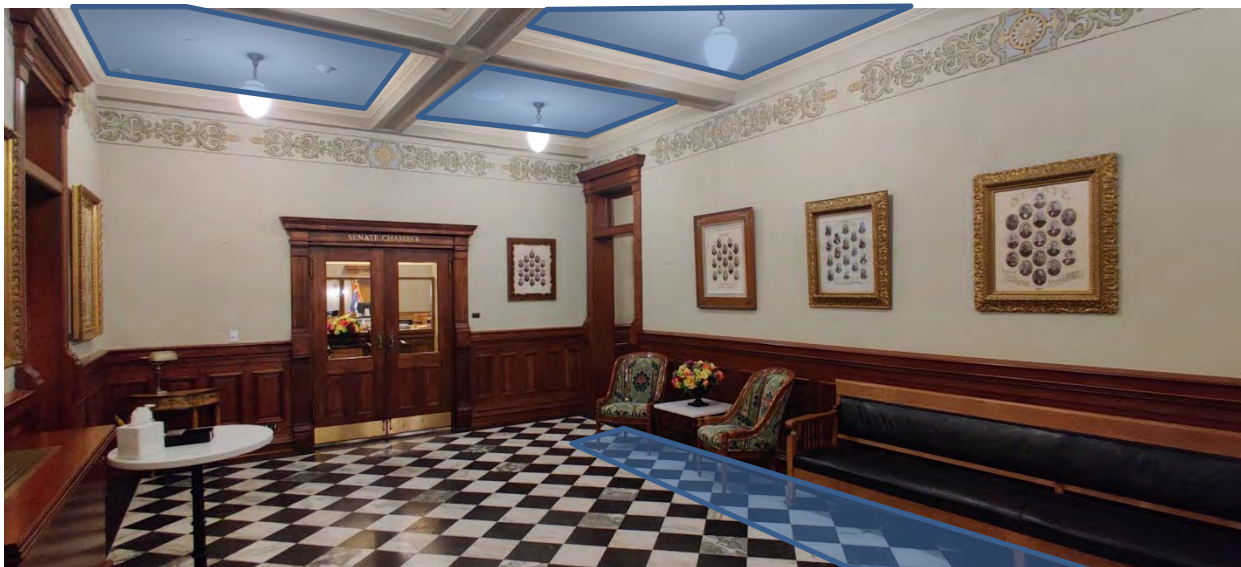
Figure 28. Recommended locations for ceiling mounted sound absorption and rugs in Senate Lobby. Layout would be similar in the House Lobby.
