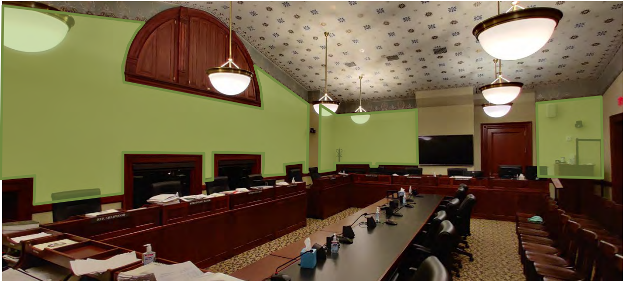
Figure 16. Recommended locations for wall mounted sound absorption. Layout would be similar on other walls not shown.
