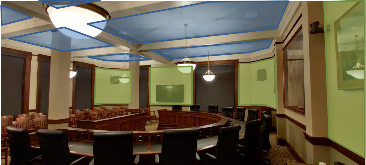
Figure 19. Recommended locations for wall and ceiling mounted sound absorption. Layout would be similar on other walls not shown. Coordination with existing architectural elements would be necessary.
