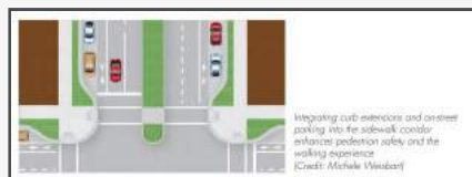
A combination of curb extensions and a median refuge narrow the roadway, reduce the pedestrian crossing distance, and reduce the time that pedestrians are in the street. Living Streets Page 5-7
