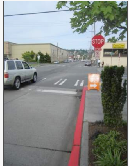
Parking restrictions at intersections may provide help pedestrians to safely cross the street by providing them with a clearer view of oncoming vehicles. Source: Peter Lagerwey.
