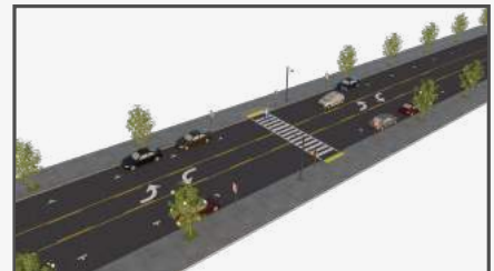
This rendering shows how the design of on-street parking can improve visibility at a midblock crosswalk. Federal Highway Administration.
